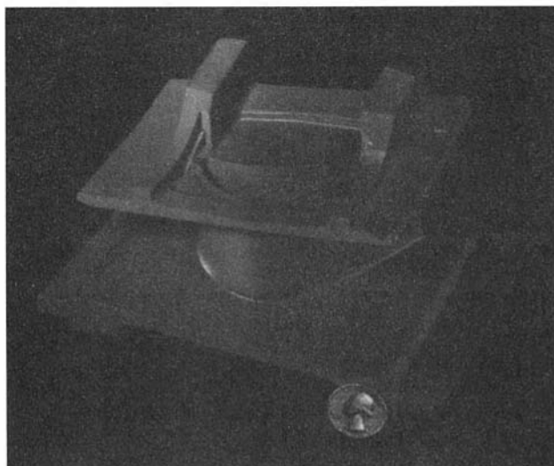
Fig. 24 Adour LP vane CMSX-4 alloy—as-cast
